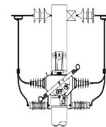
**Purpose:** This form covers the testing and commissioning of all replacements or new installations of a Nu-Lec load break switch (LBS)/sectionaliser before energisation.
