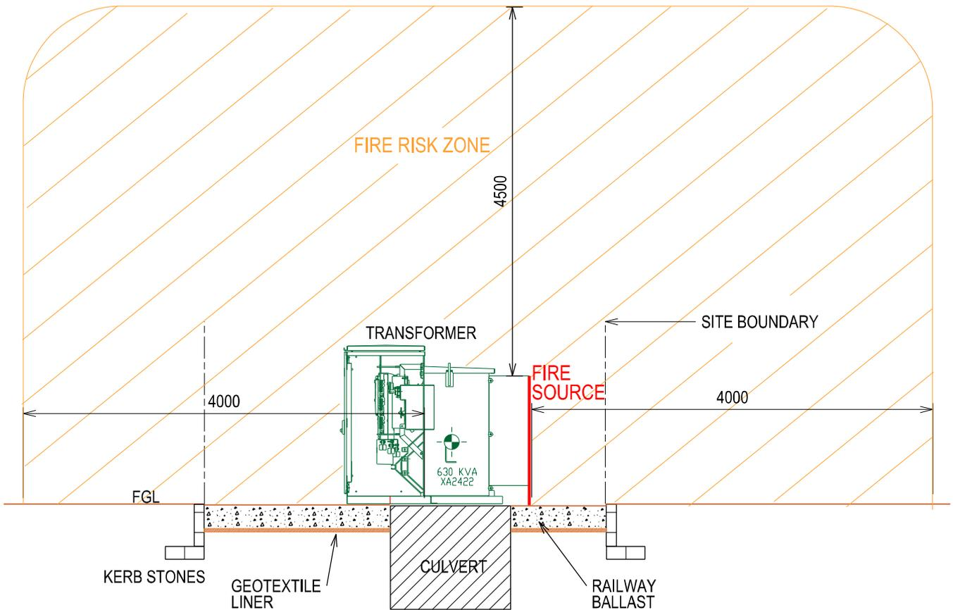
Where an oil containment bund is used, the flame trap (railway ballast) should be contained within the upper 100mm layer of the bund, sandwiched between trench covers to allow for maintenance and cleaning of the bund and replacement of the oil / water separator following an oil spill. The railway ballast is used to cool the transformer oil below its flash point as it passes through the rock into the bund below.
