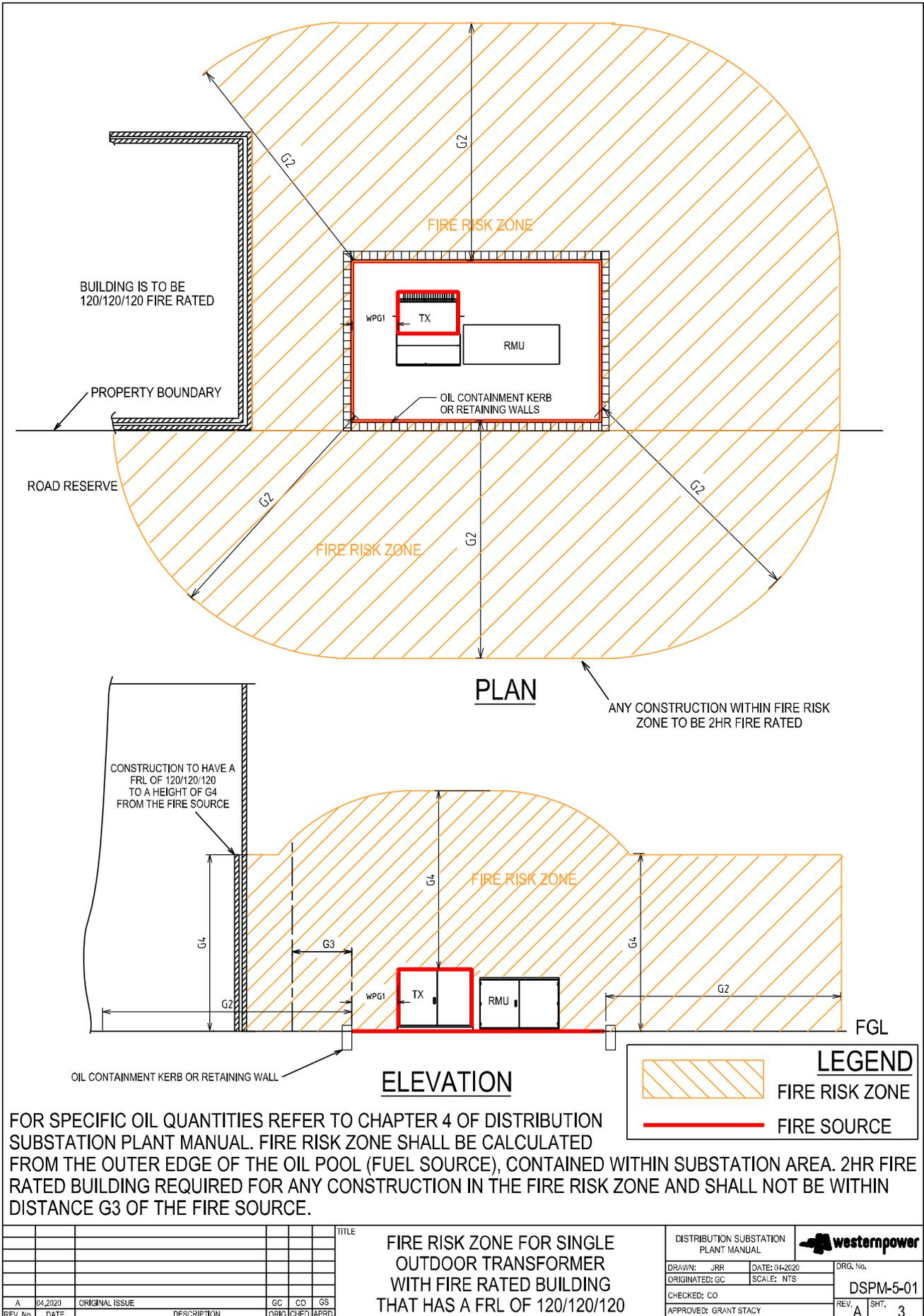
7.2 Substation Building (fire rated building example)
