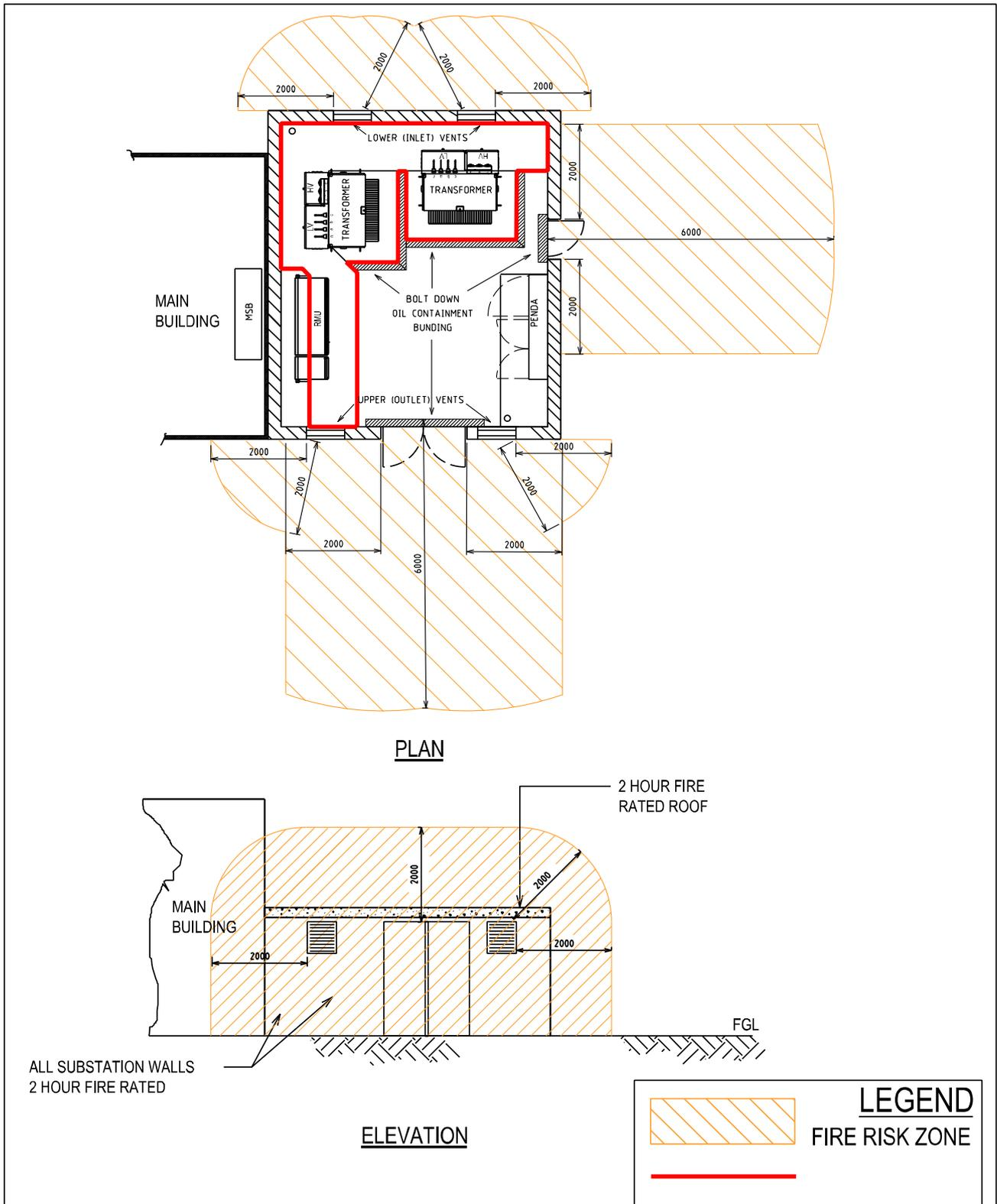
FOR SPECIFIC OIL QUANTITIES REFER TO CHAPTER 4 OF DISTRIBUTION SUBSTATION PLANT MANUAL. FIRE RISK ZONE SHALL BE CALCULATED FROM THE OUTER EDGE OF THE SUBSTATION DOORS AND VENTS. NO EMERGENCY EGRESS ROUTES PERMITTED WITHIN FIRE RISK ZONE.
