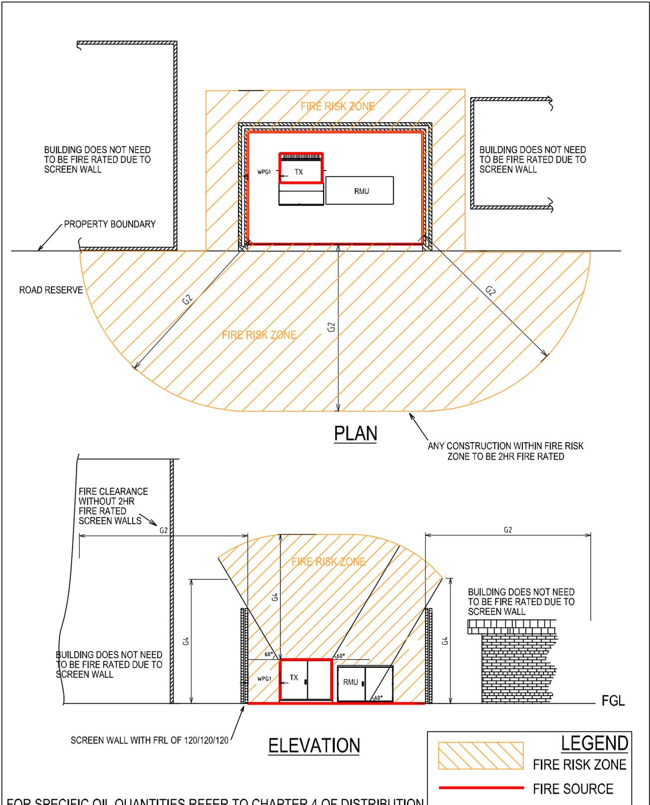
FOR SPECIFIC OIL QUANTITIES REFER TO CHAPTER 4 OF DISTRIBUTION SUBSTATION PLANT MANUAL. FIRE RISK ZONE SHALL BE CALCULATED FROM THE OUTER EDGE OF THE OIL POOL (FUEL SOURCE), CONTAINED WITHIN SUBSTATION AREA, WHEN PROJECTED AT AN ANGLE OF 60° FROM THE FIRE SOURCE ABOVE THE SCREEN WALL.
