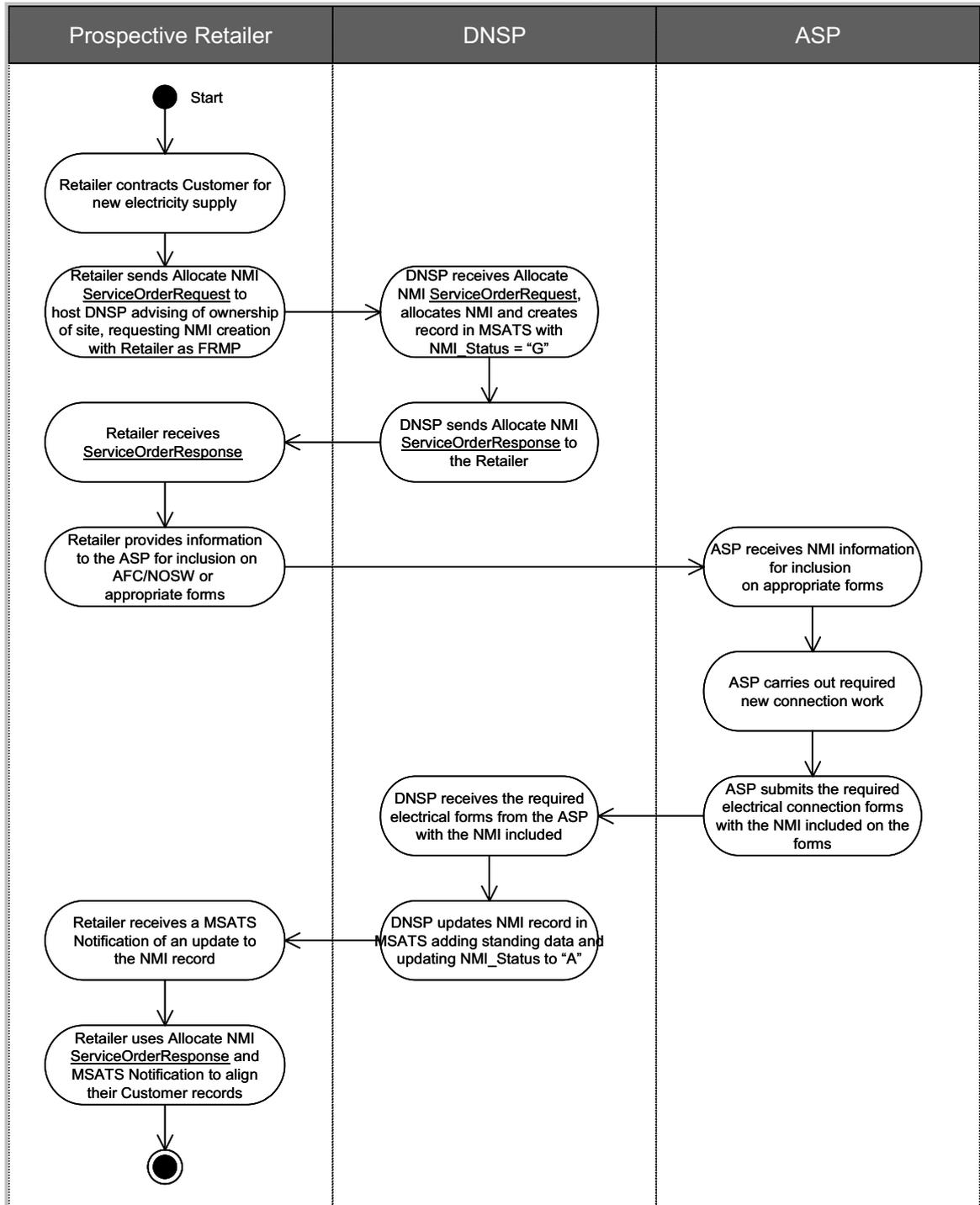
Figure 3: NSW Greenfield New Connection process
