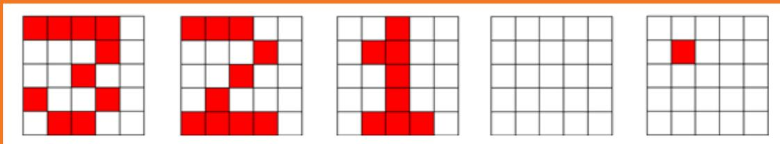
The micro:bit will display a countdown timer: 3... 2... 1... then the screen will go blank, and after a random time interval, an LED will turn on. That is the signal! Which player will react quicker?
