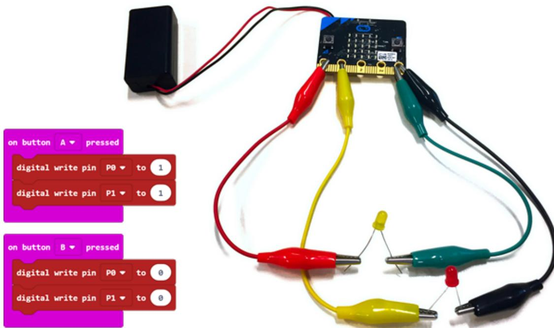
After students have made their predictions, ask them to build the circuit and test it out. Note that the minus end of the LEDs must always be connected to Ground, so the first LED will be connected to Pin 0 and Ground, the second LED will be connected to Pin 1 and Ground, and so on (this was previously explored in the extension ideas for Activity Three).
