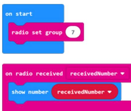
Note that the radio group number (7 in the above example) needs to be different for each group so that the micro:bits in that group can all talk to each other. The radio number can be any number between 1 and 128. The idea is similar to walkie talkies which all need to be on the same radio frequency.
