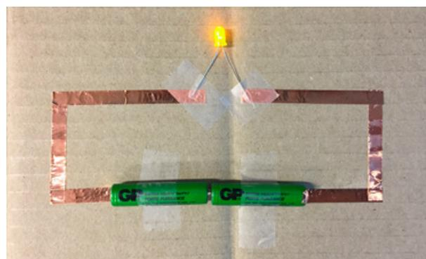
In order to provide a more engaging demonstration, teachers may wish to try making this circuit themselves prior to starting the activity with students. Note that two AAA batteries are required in order to provide sufficient voltage, and you will need to press the two batteries firmly together by hand to ensure a connection (this is why battery holders normally contain springs).
